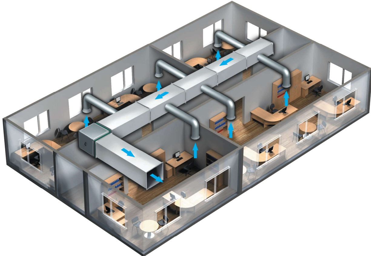
VS EC fan office ventilation example
